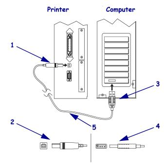
Figure 8 • Connecting the Printer through a USB Port
